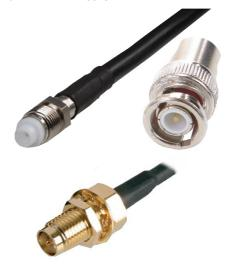
The aerial cable will be terminated with either an FME and BNC (Top Image) or SMA. Unscrew the BNC adaptor leaving only the small FME plug. The FME or SMA will pass through 8mm holes.
