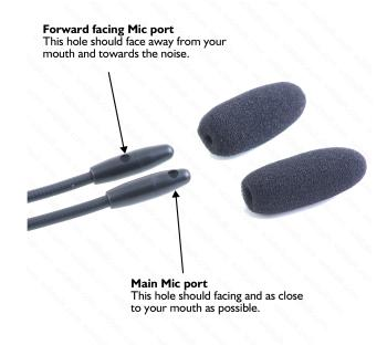
If it is reported that your voice sounds muffled it will be that a small drop of water is blocking the Mic port. A quick blow or suck on the foam is usually enough to clear the blockage.
