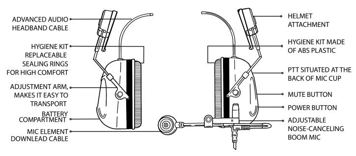
The SWATCOM 2Talk ARBORCOM Helmet Attached (AK6591) headset allows hands-free, full duplex encrypted communication between two matching headsets up to 200 meters apart
